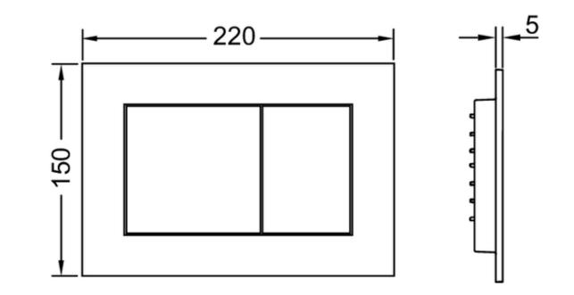
Suitable for use with all TECE Cisterns. Minimum wall thickness for button installation is 18mm (includes sheeting and tiles).
