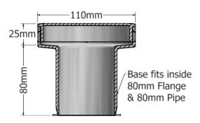
Connection to pipe must be primed and solvent welded.
