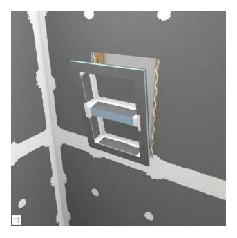
2 Fasteners each side of the niche are set to create a flush transition to the wall boards. Another 10 mm bead of wedi 610 adhesive sealant is spread over fasteners and seams.
