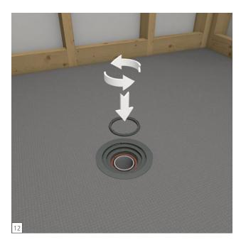
Insert the Locking Nut with notched side up into the threaded part of the Drain Unit opening and screw down until Locking Nut top is flush with top edge of Drain Unit's threaded part. Important: Turn Locking Nut to LEFT to insert and screw into flush position (turn Counter-Clockwise).
