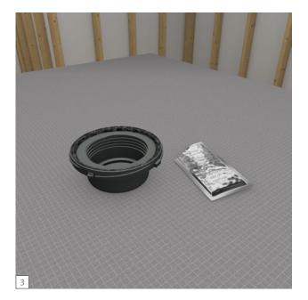
Apply the wedi provided safe Lubricant to the black rubber ring inside the wedi Drain Body.
