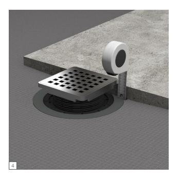
Dry-fit a tile for the shower base right next to the extended drain cover unit and determine to what height the Drain Cover Extension may need to be cut down for a drain cover top flush with the top of the tile (or drain cover top slightly below top of tile). Account for the thickness of the (compressed) tile adhesive used to install the tile.
