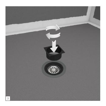
Optionally, use and insert the threaded Drain Cover Extension into the threaded part of the Alignment Ring 1. Dry fit the Drain Cover Extension for the needed final height position of the drain cover unit. The Drain Cover Extension only works for wedi's finished surface drain covers, but not with wedi's tileable covers due to their special water drainage design.
