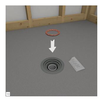
Apply wedi provided safe Lubricant to the Rubber Sealing Gasket and insert the Rubber Sealing Gasket between the wedi Drain Unit's interior and the outside of the DN50 waste pipe in the floor. Push the Rubber Sealing Gasket down along the waste pipe until it is stopped by the Drain Unit's lower interior flange.
