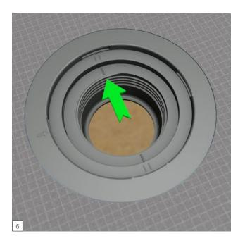
On the top side of the drain you can also verify the drain unit has successfully connected when the single hash marks are centered between the double hash marks.
