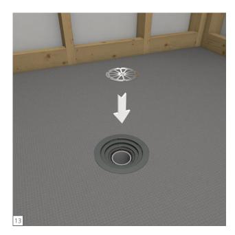
Insert Strainer Key into Locking Nut at notch connections and with Strainer Key printed side up. The Strainer Key is used as a tool to tighten the compression seal of the Drain Unit, but remains in place later to serve as a hair catcher to protect the drain and make maintenance and cleaning easy.
