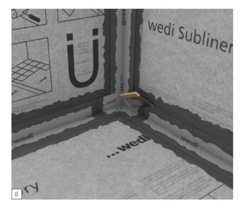
wedi Tools sealing corners and wedi Tools sealing gaiters are used for internal and external corners as well as pipe penetrations.
