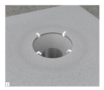
Push the sides of the gaiter firmly towards the drain.
