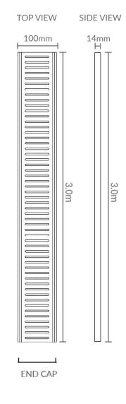
\* Total length of full grate is 3.2m, total usable length is 3m to allow for any wastage during the anodising process.
