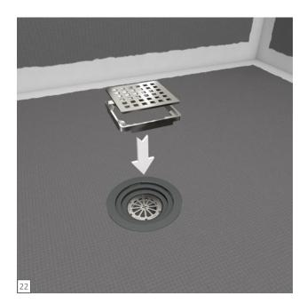
You can now insert the drain cover unit consisting of a stainless steel frame and the stainless steel cover itself. The drain cover unit fits in loosely and the drain installation is complete.
