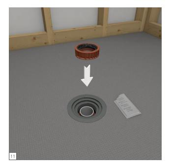
Apply wedi provided safe Lubricant to the rubber part of the Compression Spacer. With the rubberized part pointing up now insert the Compression Spacer in between Drain Unit and waste pipe and on top of the Sealing Gasket. The Compression Spacer will push the Rubber Sealing Gasket down into its resting position.
