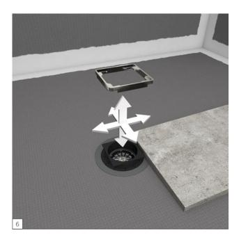
Place the drain cover unit loosely on the Drain Cover Extension were it fits into a tight seat. The cover is now vertically adjustable and can also move horizontally to fit the tile layout.
