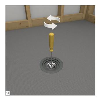
Insert a flat headed screwdriver into Strainer Key slit and turn **LEFT** to tighten the compression seal (turn Counter-Clockwise). Achieve a hand-tight fit and do not over-tighten.
