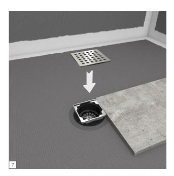
The drain cover unit can still be moved laterally 3/16 in. in either direction, and can be aligned with the tile.
