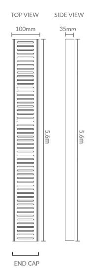
\* Total length is 5.8m, total usable length is 5.6m to allow for any wastage during the anodising process.
