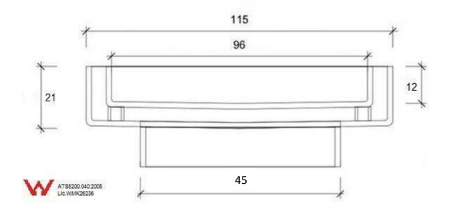
BT CODE: 1264410 SUPPLIER CODE: KFG-845G DESCRIPTION: Tile Insert Floor Drain
