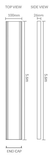
\* Total length of full grate is 5.8m, total usable length is 5.6m to allow for any wastage during the anodising process.
