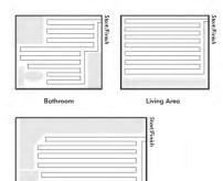
Try and leave the longest wall to last. That way if you have a little too much or too little cable left you can make an easy adjustment by coming a bit further away or going right up close to the wall. Neither option will affect the heating of the room in any way.
